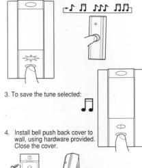
Note: Before final installation, adjust distance and position between push and chime to optimize the chime within your environment. Dense walls and metal can reduce range.
