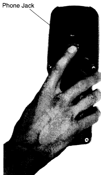
Phone Jack on rear of Dolphin 7400
