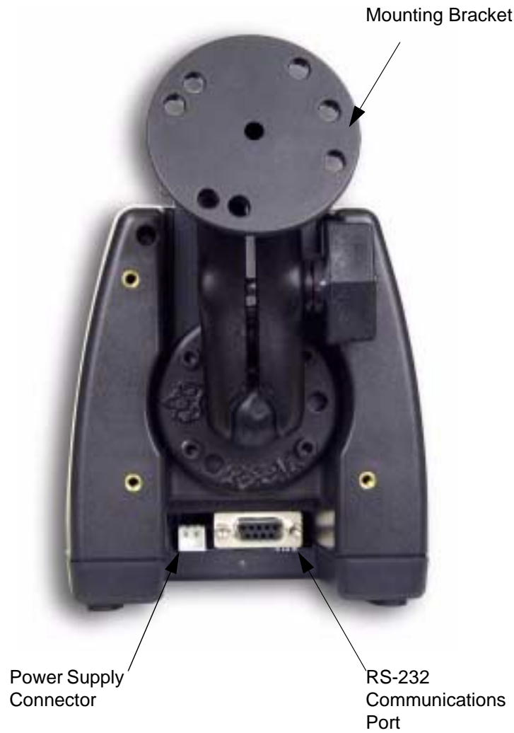
Rear Panel of Dolphin Mobile IntelliBase
