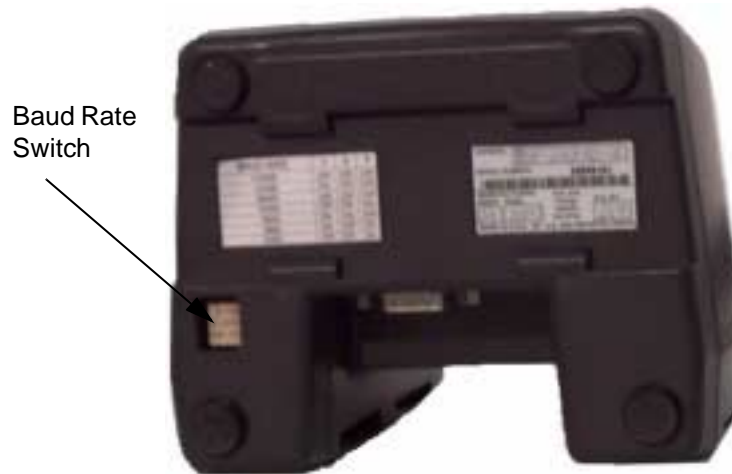
Bottom View of HomeBase/IntelliBase
