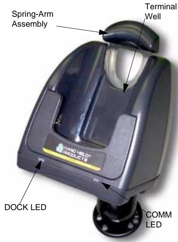
Front Panel of Dolphin Mobile IntelliBase
