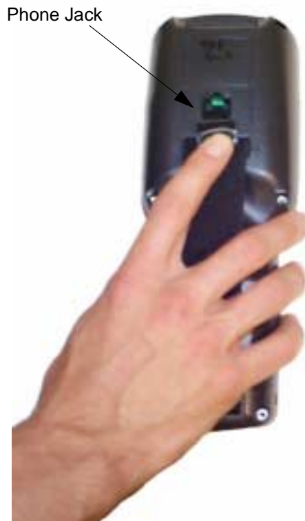
Phone Jack on rear of Dolphin 7400
