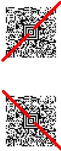
The aiming beam is smaller when the terminal is held closer to the code and larger when it is farther from the code. Symbologies with smaller bars or elements (mil size) should be read closer to the unit. Symbologies with larger bars or elements (mil size) should be read farther from the unit.
