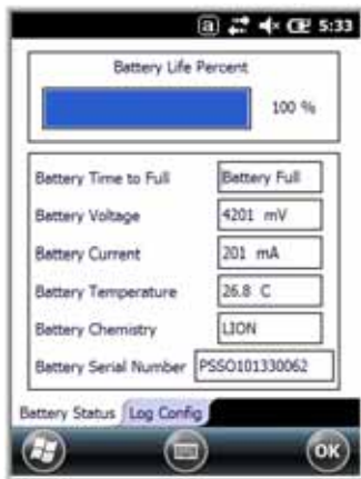
Battery Status Tab
