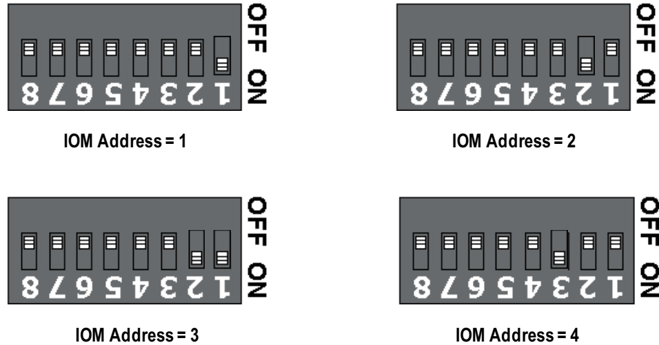
Fig. 32. IOM Address set up - S3 Settings
