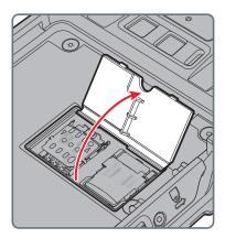
**6** Press down and slide the SIM door toward the top of the CT50 to open it.
