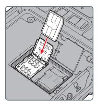
8 Close the SIM card door and slide it toward the bottom of the CT50 to secure it.
