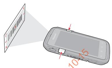
Make sure the entire bar code is inside of the frame. When the scanner successfully reads a bar code, you hear a high beep and the Good Read LED turns on briefly
