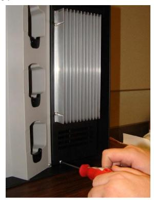
3. Pull the power supply straight out by holding onto the heat sink.
