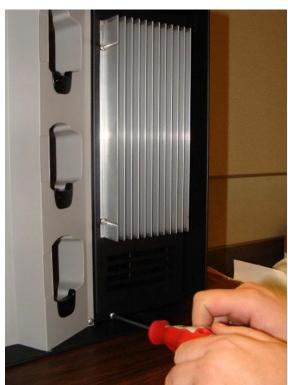
3. Pull the power supply straight out by holding onto the heat sink.
