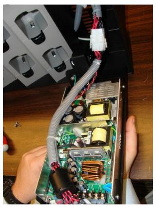
17. Using the heat sink, place the power supply back into the main unit.
