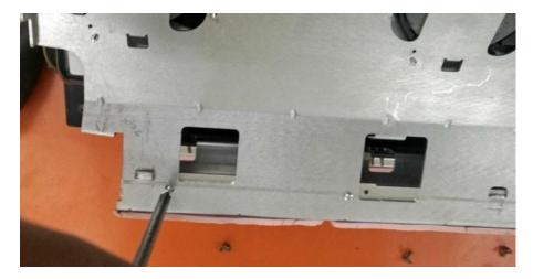
4. Remove the **black** screws between the frames and plastic bay cover.
