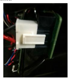
Disconnect the power supply harness from the power distribution board and set the bays aside in a clean work area.
