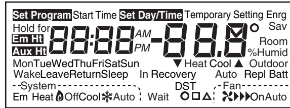
Fig. 10. Display of all the segments of the LCD.
