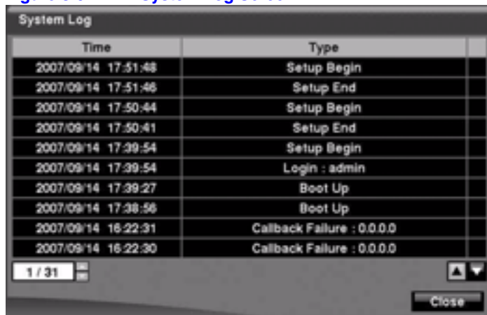
Figure 3-9 System Log Screen
