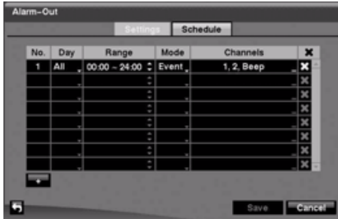
Figure 3-39 Alarm-Out Schedule Screen
