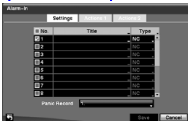
Figure 3-51 Alarm-In Settings Screen
