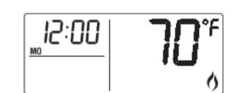
stat. The thermostat will display the ambient temperature once it is installed on the wall. By default, the setpoint is 70°F (21°C).
