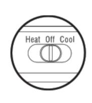
**Note**: When you place the thermostat in Cooling mode, you might need to wait up to five minutes before cooling can start. This is a safety feature for the compressor. \*\*will flash on the screen until cooling can start again.
