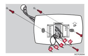
Drill 3/16-in. holes for drywall Drill 3/32-in. holes for plaster
