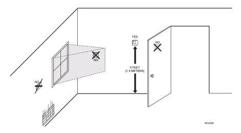
Fig. 1. Typical location of thermostat.
