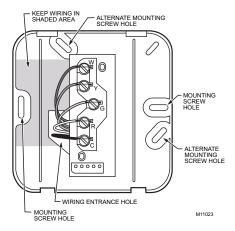
Fig. 3. Restrict wiring to shaded area.
