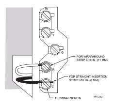
Fig. 4. Wiring connections.
