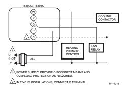
Fig. 5. T8400C/T8401C heat-cool wiring diagram in single transformer system with gas heat/electric cooling.
