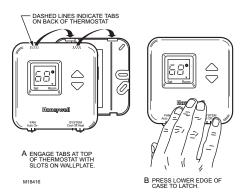
Fig. 7. Mounting thermostat wallplate.
