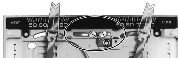
NONADJUSTABLE STOPS WITH LOCKING LEVER SCREWS 75°F (24°C) MAX. HEAT 75°F (24°C) MIN. COOL
