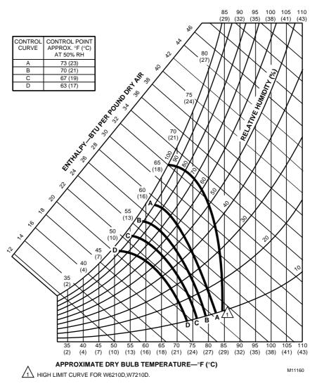
Fig. E-7. Partial psychometric chart for a C7400A Solid State Enthalpy Sensor.
