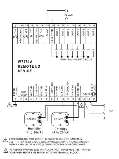
Fig. 17. Typical Humidity and Enthalpy (4 to 20mA) sensor wiring diagram. (For note 2, refer to Fig. 15.)
