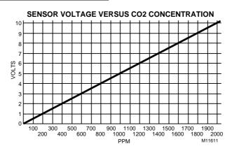
Fig. E-9. Graph of Sensor Voltage versus CO<sub>2</sub> concentration.
