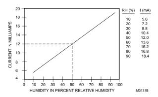
Fig. 5. C7600C output current vs. humidity.
