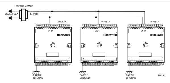
Fig. 13. Power wiring details for two or more Excel 10s per transformer.
