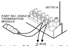
(B) Installing E-Bus Termination Module & W7761A
