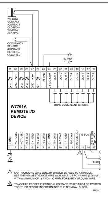
Fig. 18. Typical Window and Occupancy sensor wiring diagram. (For note 2, refer to Fig. 15.)
