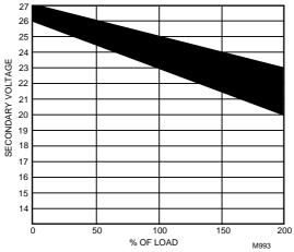
Fig. 11. NEMA class 2 transformer voltage output limits.
