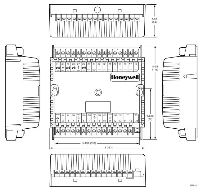
Fig. 4. W7761A construction in in. (mm).
