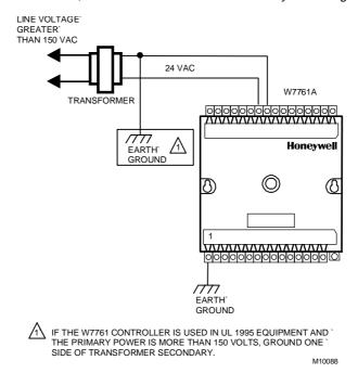
Fig. 14. Transformer power wiring details for one Excel 10 used in UL 1995 equipment (U.S. only).
