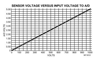
Fig. E-10. Graph of Sensor Voltage versus input Voltage to A/D.
