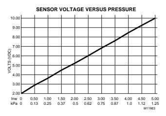
Fig. E-11. Graph of Sensor Voltage (Vdc) versus Pressure (Inw).
