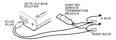
(F) Twist wires and attach wire nuts to RJ-45 Adapter cables, E-Bus segment wires and Termination Module to connect to a Q7751A,B Router
