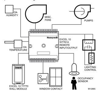
Fig. 2. Typical W7761A control application.
