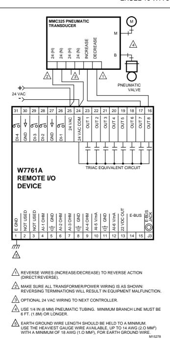
Fig. 20. Typical Pneumatic transducer (Series 60 - Floating) to W7761A.
