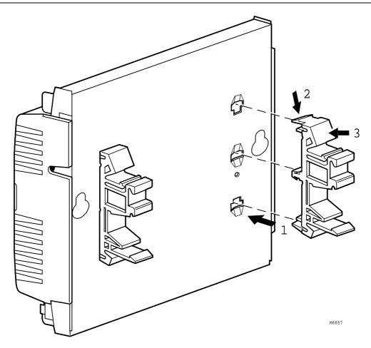
Fig. 5. DIN rail adapters.
