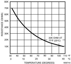
Fig. 23. Temperature sensor resistance plots.
