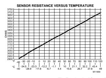
Fig. E-1. Graph of Sensor Resistance versus Temperature.
