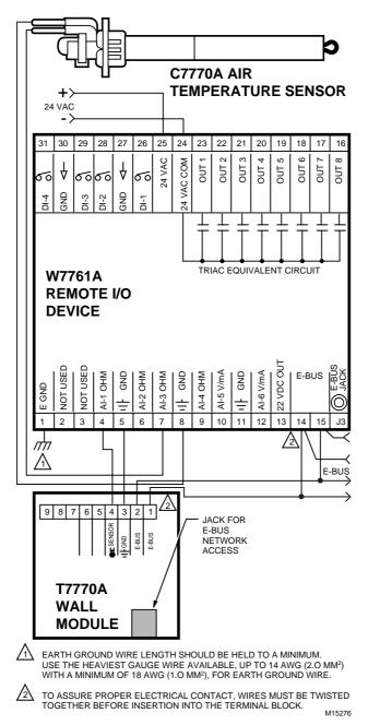
Fig. 16. Typical T7770A and C7770A wiring diagram. (For note 2, refer to Fig. 15.)
