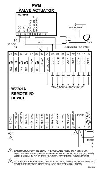
Fig. 19. Typical PWM Valve Actuator and miscellaneous fan control to W7761A. (For note 2, refer to Fig. 15.)
