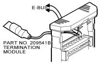
INSERT INTO TERMINALS 1 AND 2 WITH THE E-BUS WIRE. TERMINATION MODULE IS PHYSICALLY LOCATED BEHIND THE T7770 INSIDE THE 2 X 4 OR 60 MM BOX.
