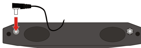
Figure 18 Connect External Power Supply
