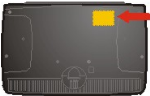
Figure 1 CDRH / IEC 825 Caution Label Location – MX3X, Back
