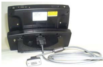
Figure 41 ActiveSync Cable Connected to Serial port on Cradle
