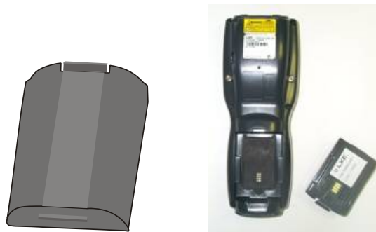
Figure 10 Main Battery Pack
