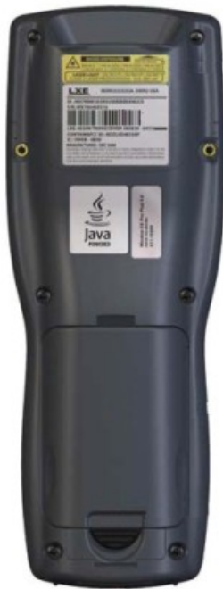
Figure 1 CDRH / IEC 825 Caution Label Location – MX8, Back
