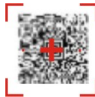
Figure 24 Imager Bracketed Crosshair Target on 2D Barcode
