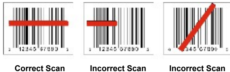
Figure 23 Laser Scanner Beam on Linear Barcode
