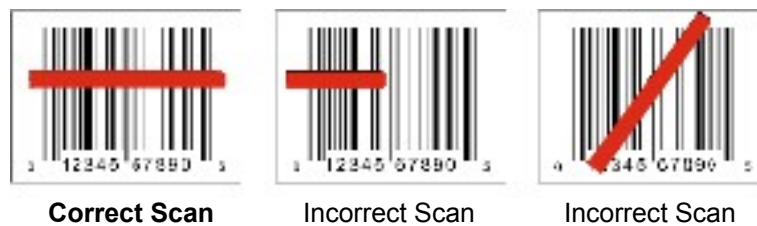
Figure 26 Laser Scan Beam on Linear Barcode
