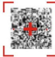
Figure 27 Imager Bracketed Crosshair Target on 2D Barcode
