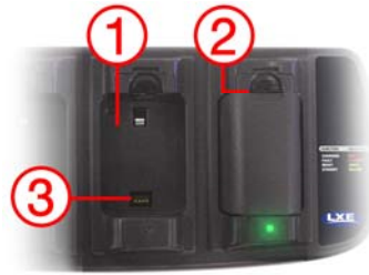
Figure 39 Insert Battery Pack in Charging Pocket
