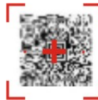
Figure 29 Imager Bracketed Crosshair Target on 2D Barcode
