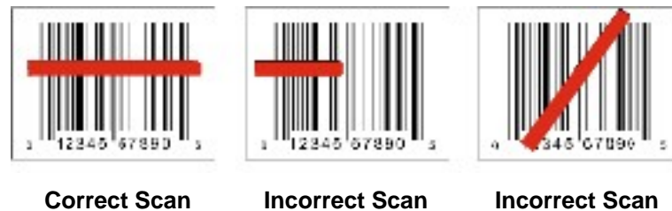
Figure 28 Laser Scanner Beam on Linear Barcode
