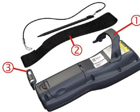
Figure 15 Attaching the Handstrap
