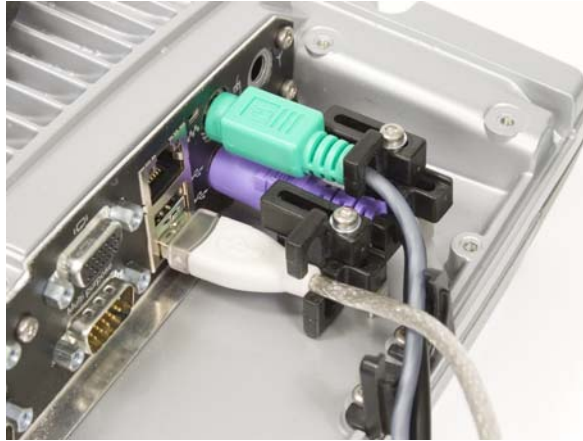
Figure 8: Strain relieving brackets for USB and PS/2 connectors
