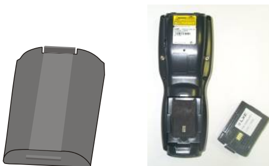
Figure 8 Main Battery Pack
