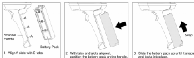
Figure 7. Steps for Installing the Battery
