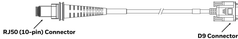
1. Seat the D9 connector of the cable over the USB or USB11 connector on the dock.
