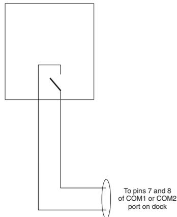
Pins 7 and 8 must be connected as shown in the illustration above. No other pins are to be connected.
