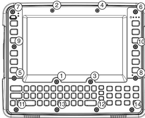
6. Carefully lift the front panel away from the device.
