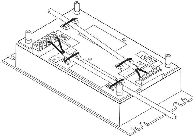
8. Route the wiring from the DC/DC power supply to the vehicle's electrical system. Do not connect to vehicle power at this time.
