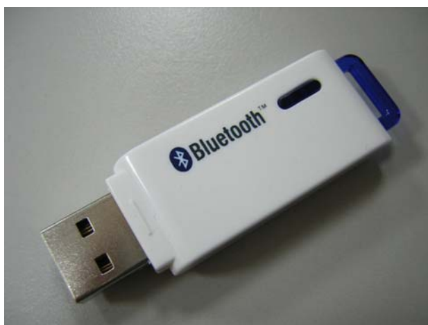
Figure 1-9: USB Bluetooth Adapter
