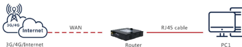
Figure 3-1 Single Equipment Direct Connection
