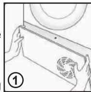
2. Turn the two locking levers anti-clockwise and pull out the front cover.
