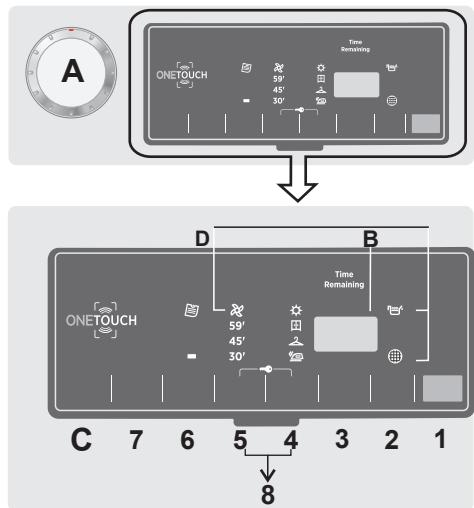
**A-Programme Selector** - Rotating the knob in both directions it's possible to select the desired drying program. To cancel the selections or switch off the dryer rotate the knob on OFF.
