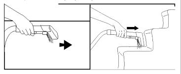
With cleaner placed on a stable surface, pre-spray a small area of carpet or carpeted stair by holding the nozzle about one inch above the carpet and push it forward while pressing the trigger (equals one wet stroke).
