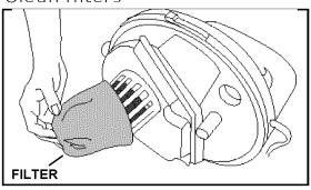
**d**. Remove debris from recovery tank filter and rinse with clean water. Filter may be removed for cleaning.
