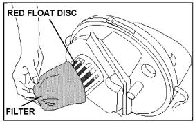
When the recovery tank is full, the automatic "shut-off" mechanism will turn off the cleaner suction.
