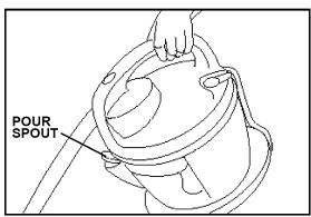
Empty tank by pouring dirty solution from pour spout.
