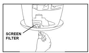
**f**. Remove debris from screen filter located at bottom of cleaner. Be careful not to poke through screen filter when cleaning.
