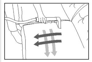
For heavily soiled areas, it may be necessary to repeat the cleaning process. Make criscrossing strokes to the original pattern; overlap each pass.
