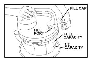
Remove fill cap. For a **full tank** of cleaning solution, pour **2 oz. of detergent** into tank through fill port and fill tank to **"full capacity"** line (1/2 gallon) with hot tap water.
