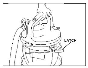
**c**. Unlatch cleaner lid by pulling latches outward on both sides of cleaner. Lift off lid.
