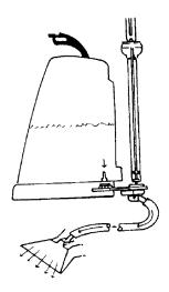
The reservoir assembly is opened by actuating the trigger in the handle.
