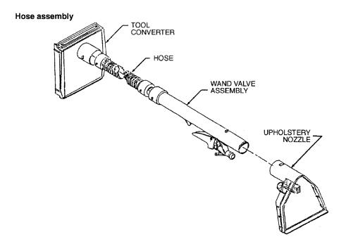
Serviceable components of the hose assembly are shown in the above diagram.
