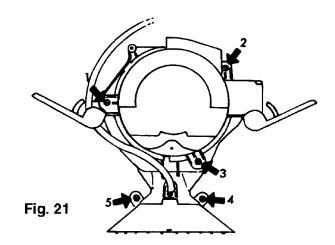
On pump models, if pump is removed, screw five will already be out.
