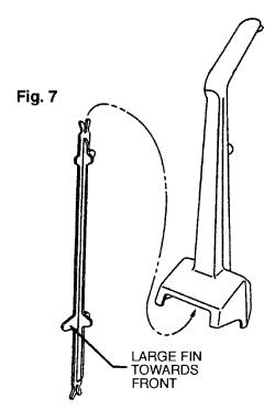
Slide it up into the handle until it snaps into position.
