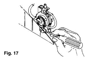
Pump is replaced as an assembly which includes the quick connect and tubing. (Fig. 18)
