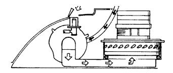
The Pump gets a constant flow of solution from the solution tank through the reservoir assembly. On models without the pump, the pump tap on the reservoir is plugged.
