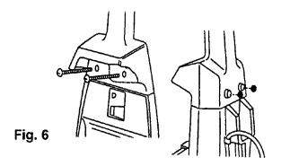
The handle is replaced as an assembly
