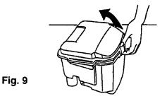
The lid is carried in service as an assembly that includes the lid, float retainer, float and filter.
