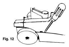
**1.** Lift hood until it clears latches and push forward to remove.
