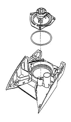
With motor cover removed disconnect leads and lift motor out of main body.
