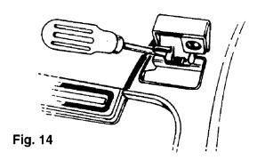
The door is replaced as an assembly (door, seal and speed nut).
