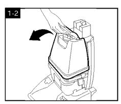
Attach upper handle Remove clean solution tank (upper tank) from deep cleaner.
