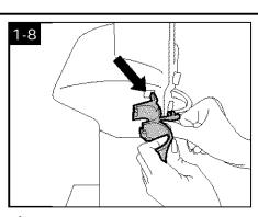
Attach hose clip Push tab on side of clip into hole on side of handle.
