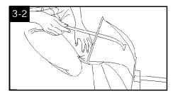
Some models have a nozzle clean-out tool for removing debris or if a non-carpeted floor is not available. To use the tool: Disconnect deep cleaner from electrical outlet. Slide tool into nozzle and remove debris as shown.
