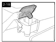
To remove tank lid, lower handle completely toward back of tank and lift off lid.
