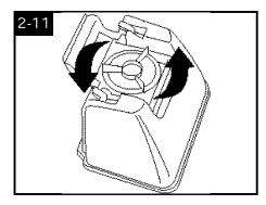
Rotate tank cap counterclockwise and lift up to remove cap.
