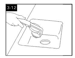
3. Drain hose by turning deep cleaner ON and holding end of hose up for several seconds. Do not press trigger.
