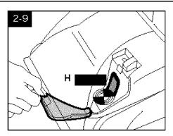
To clean screen (H), turn deep cleaner off and disconnect from electrical outlet.
