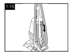
Slide bare floor attachment into holder as shown.
