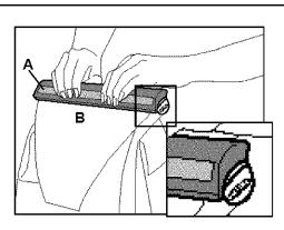
2. With foam strip (A) (located under the netting) in position as shown, place attachment on front of nozzle (B). Make sure arrow on end of attachment points in the direction as shown.
