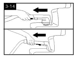
9. Lift tool, and position it against riser. Pull tool **slowly** over carpet without pressing trigger (dry stroke).
