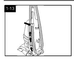
Then continue wrapping hose as shown snapping end of hose connector into clip.
