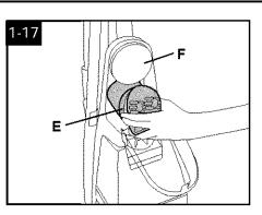
To remove powered hand tool (E), pull it down and outward.
