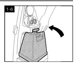
Replace clean solution tank (upper tank) by positioning bottom first. Press on tank handle to snap top of tank into place.
