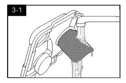
**d.** Remove debris from recovery tank filter and rinse with clean water.
