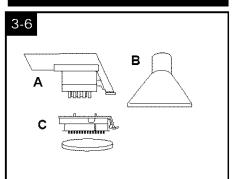
**A. Powered hand tool** has rotating brushes for extra scrubbing action on small carpet areas, carpeted stairs and upholstery. Brushes can be removed for converting to the scrub module.
