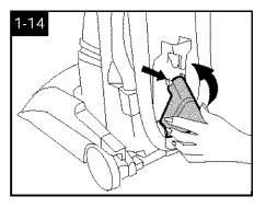
Position tool in holder at base of cleaner and snap it into place as shown at arrow.
