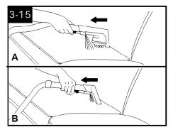
6. Gently press the tool (A) or (B) onto the fabric. Press the trigger and slowly pull the nozzle over the fabric.
