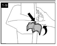
Pivot clip and push other tab into hole at back of handle to lock into place.
