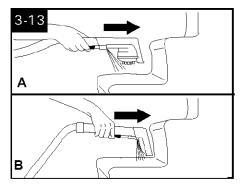
7. Pre-spray the carpeted stair by holding the tool (A) or (B) about one inch above the carpet and push it forward while pressing the trigger (equals one wet stroke).
