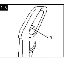
When handle sections are completely together, squeeze trigger (B) on upper handle to snap trigger rod In place.
