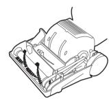
Remove brush assembly and check for wear on the belt. Loop the new belt around the motor and brush assembly.
