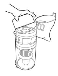
Separate the GREY foam filter from the BLUE HEPA filter pack using the tab provided.
