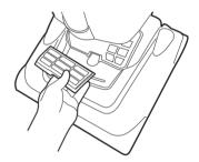
Wash the exhaust filter under hand warm water until the water runs clean. Remove excess water by shaking and leave to dry for 24 hours. Refit filter only when completely dry. DO NOT USE HOT WATER OR DETERGENTS.
