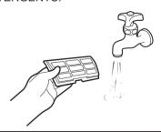
**IMPORTANT!** For optimum performance, always keep your filters clean. We recommend that the exhaust filter should be washed every 3 MONTHS.
