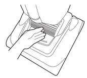
Remove the exhaust filter.
