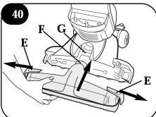
Return cleaner to upright position. Replace nozzle, making sure latches (E) are out.
