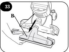
Remove nozzle (B) by pulling straight out.
