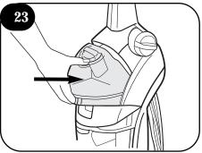
Slide tank straight into position until latch snaps in place.
