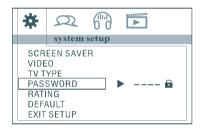
Enter the password and press ENTER button. Type the old password (The initial factory code is 0000) Enter the 4 character password that you want to use . Type again to confirm password.
