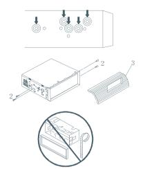
Installation using the screw holes on the sides of the unit.
