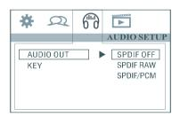
This is to activate the audio output from SPDIF OFF mode to SPDIF RAW mode or SPDIF PCM mode.
