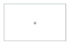
Aim at the "+" and tap it, the symbol will moves around the touch screen, tap it six times, system will finish calibration automatically and exit calibration mode.
