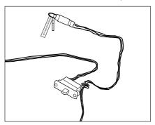
After you've programmed your model it's important to rebind the system so the true low throttle and neutral control surface positions are programmed.
