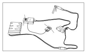
Turn on the receiver switch. Note that the LED's on both receivers should be flashing indicating that the receiver is ready to bind.
