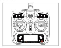
Press and hold the bind button on the back of the transmitter while turning on the power switch. The bind button should flash and within a few seconds the system should connect. The LED's on the receivers should go solid indicating the system has connected.
