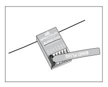
Power on the receiver. If the receiver is installed in an electric aircraft, turn on the speed controller to power up the receiver. If the receiver is going to be powered by a separate battery, plug the battery into any unused port. The amber light will blink, indicating the AR6100 is in bind mode.
