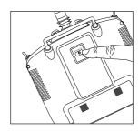
**IMPORTANT**: Remove the bind plug to prevent the system from rebinding the next time the power is turned on.
