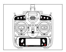
Press and hold the bind button on the back of the transmitter while turning on the transmitter. The button will flash for several seconds, then the LED on the transmitter and receiver will remain solid on, indicating a successful bind.
