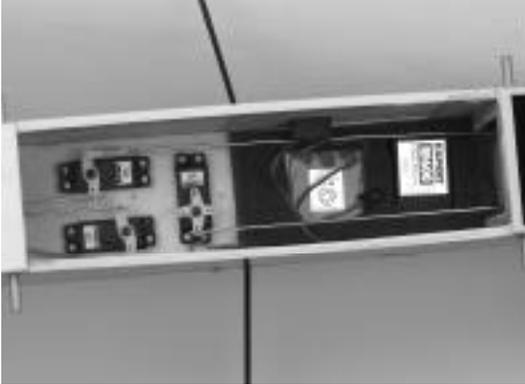
Fuselage Servo, Receiver, Battery Installation
