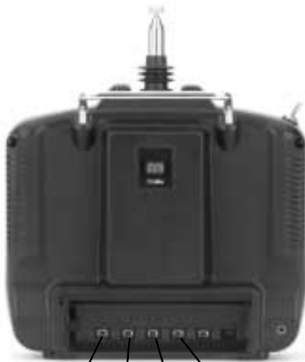
Throttle Aileron Elevator Rudder
