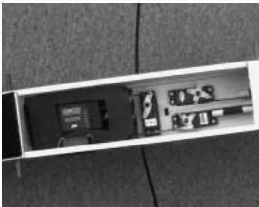
Fuselage Servo, Receiver, Battery Installation
