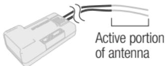
**NOTICE:** Do not cut, kink, or modify the antennas. Damage to the coaxial portion of an antenna will reduce the performance of the antenna. Shortening or cutting off the 31mm tip will reduce the range.
