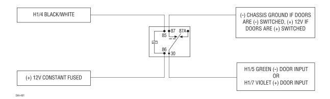
**IMPORTANT!** This output is only intended to drive a relay. It cannot be connected directly to the domelight circuit, as the output cannot support the current draw of one or more bulbs.
