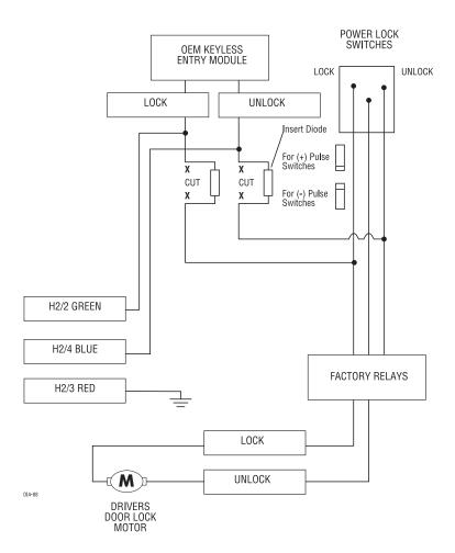
**NOTE:** Failure to insert the diodes at the correct point will allow the system to be disarmed by one of the power door lock switches inside the vehicle. The best place to insert the diode is at the keyless entry module itself or at the relays.
