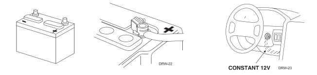
**IMPORTANT!** Do not remove the fuse holder on the RED (H1/11) wire. It ensures that the control module has its own fuse, of the proper value, regardless of how many accessories are added to the main power feed.
