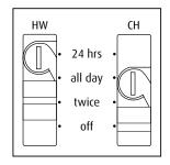
**Gravity -** On this type of system it is possible to have hot water without central heating, but not central heating without hot water. In this case the installer would have interlocked the select switches as illustrated on the right.
