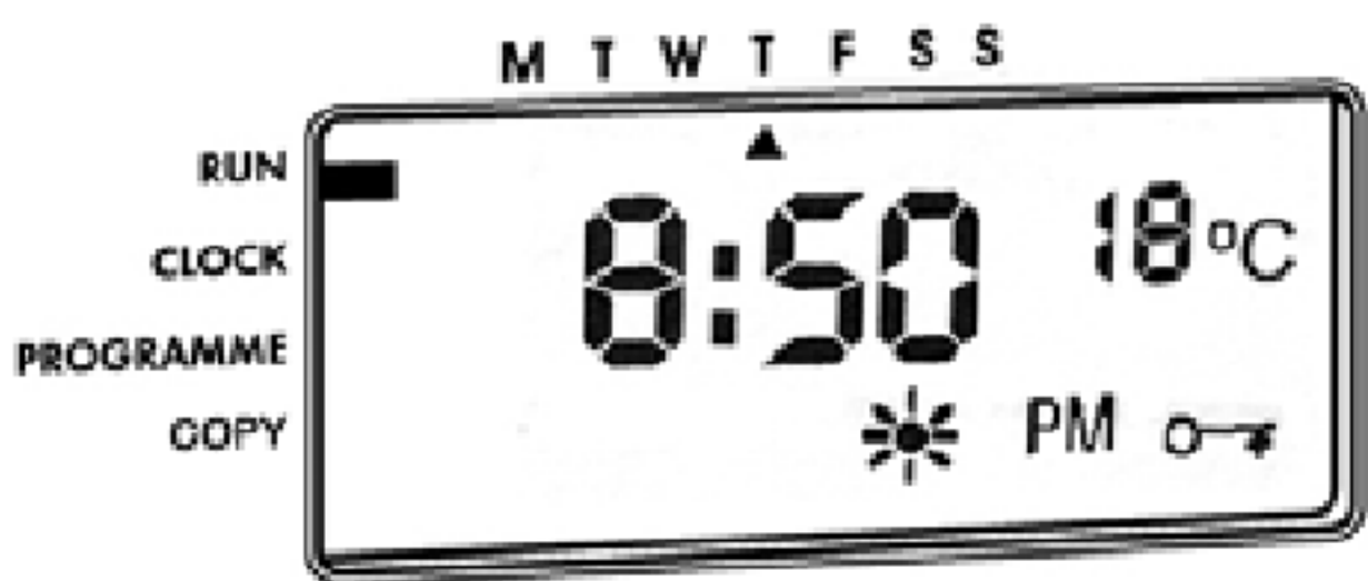
Display 1 - Shows current time and target temperature
