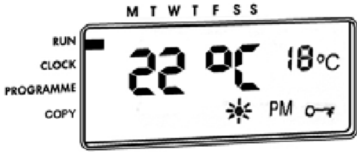
Display 2 - Shows current and target temperature
