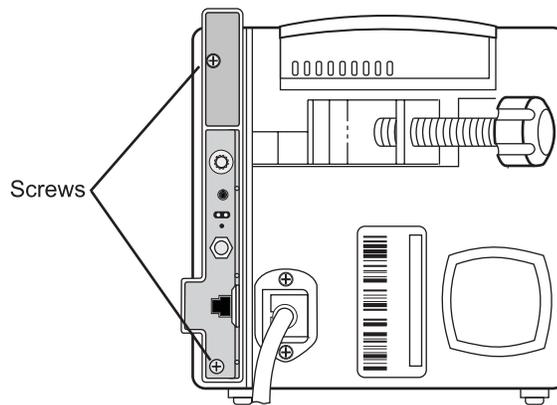
**Figure 1. Remove Screws**
