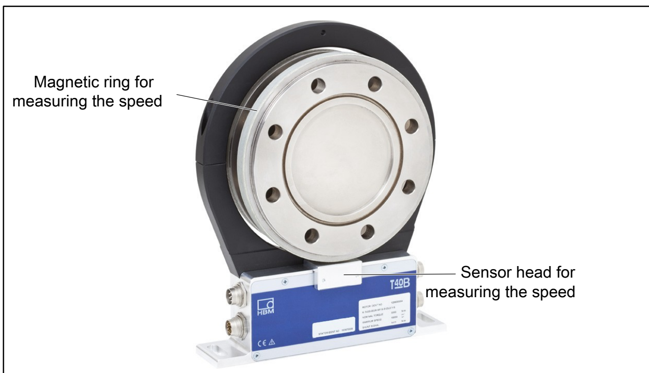
Fig. 5.15: Torque transducer with speed measurement
