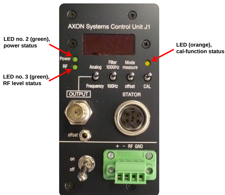
Fig. 8.1: LEDs on the evaluation unit
