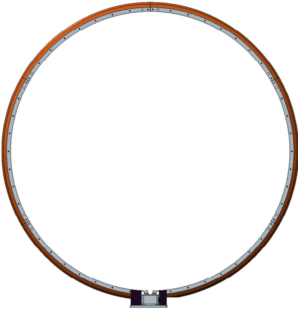
Fig 4.2: Mechanical construction of stator with mounted shielding
