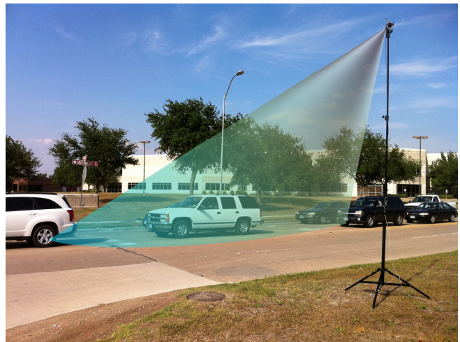
Illustration of rotated PD300 in side-firing intersection mode with maximum width of view.
