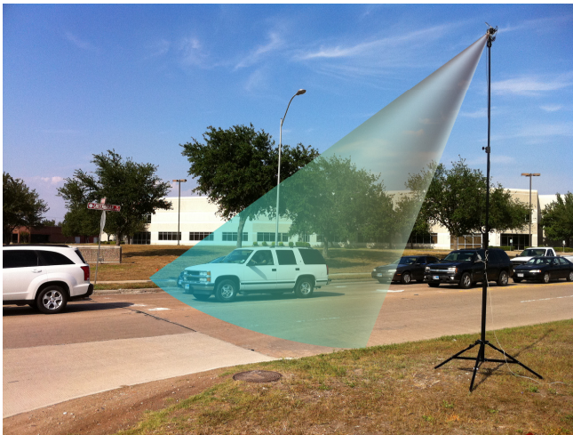
Illustration of PD300 in side-firing intersection mode with maximum depth of view.
