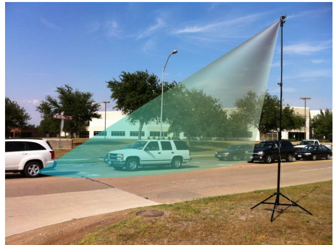
Illustration of rotated PD420 in side-firing intersection mode with maximum width of view.
