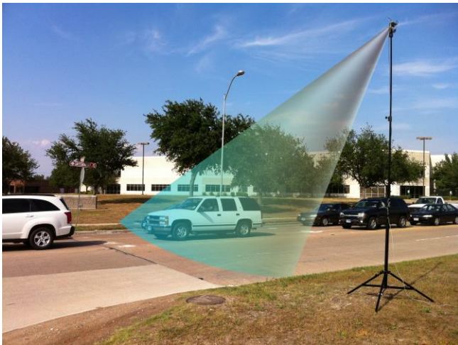
Illustration of PD420 in side-firing intersection mode with maximum depth of view.
