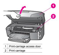
3 When the print carriage is idle and silent, press down and then lift a latch inside the HP all-in-one.
