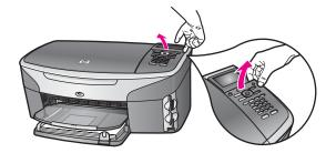
Tip You can also use a thin, flat object, such as a credit card, to lift the control panel overlay. Gently slide the credit card at a slight angle, about 45 degrees, between the color graphics display and the control panel overlay. Apply slight downward pressure to lift the control panel overlay.
