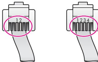
If you used the 4-wire phone cord, disconnect it, find the supplied 2-wire cord, and then connect the 2-wire cord to the port labeled "1-LINE" on the back of your HP all-in-one. For more information on connecting this phone cord and setting up your HP all-in-one for faxing, see [Fax setup](#). If the supplied phone cord is not long enough, you can extend it. For information see [The phone cord that came with my HP all-in-one is not long enough](#).
