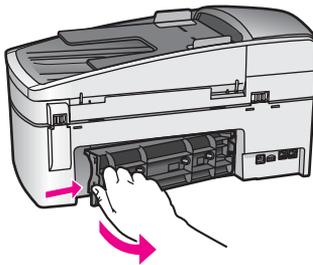
**Caution** Trying to clear a paper jam from the front of the HP all-in-one can damage the print mechanism. Always access and clear paper jams through the rear clean-out door.
