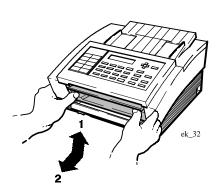
To clear a paper jam: Lift and remove the paper delivery tray. Do not attempt to clear paper from the print cartridge area.
